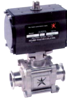
SERIES 77SN Direct Mounting Design Size: 1/2" - 4" True Tube Full Port Body, Ends: CF3M Ball: CF3M / 316L S/S Stem: 316L S/S Seats: PTFE Rating: 1000 PSI max.
